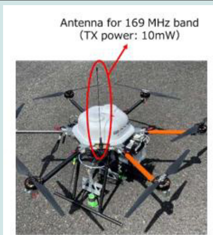
(b) Repeater and mission drone. Figure 7: Antenna installation.
