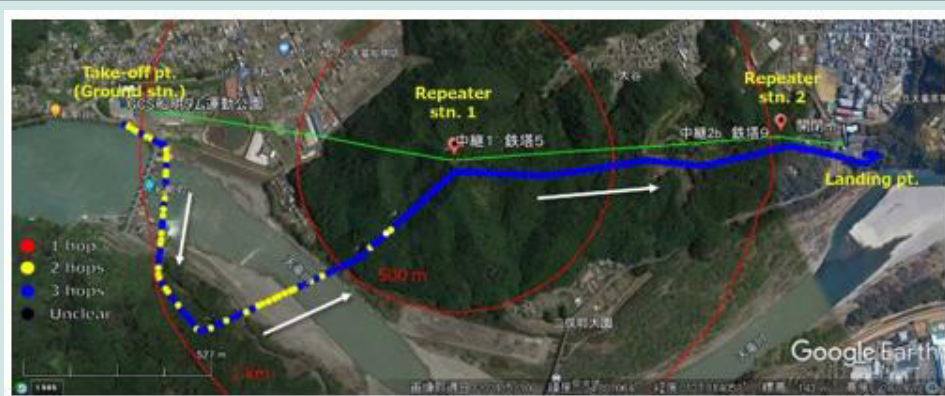
Figure 16: The change of the number of hops along with the flight location.
