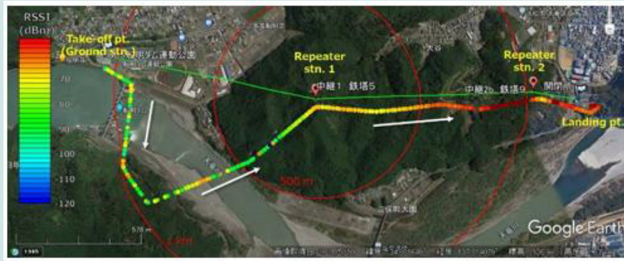
Figure 17: The change of the receiving signal power at the terminal station along with the flight path.
