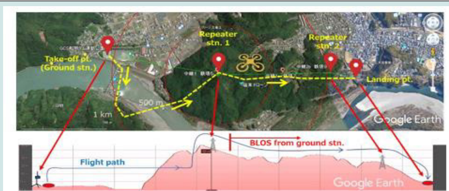
Figure 14: The location of each station, the terrain profile and the flight path.
