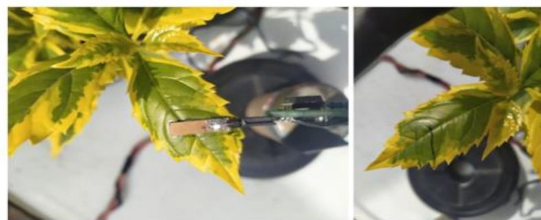
Figure 4: Ornamental plant with capacitor sensor.
