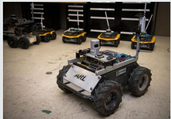
**Figure 1:** Illustrates a small unmanned Clear path Husky robot, which was used by ARL researchers to develop a new technique to quickly teach robots novel traversal behaviors with minimal human oversight. Image Credit: US Army [2].
