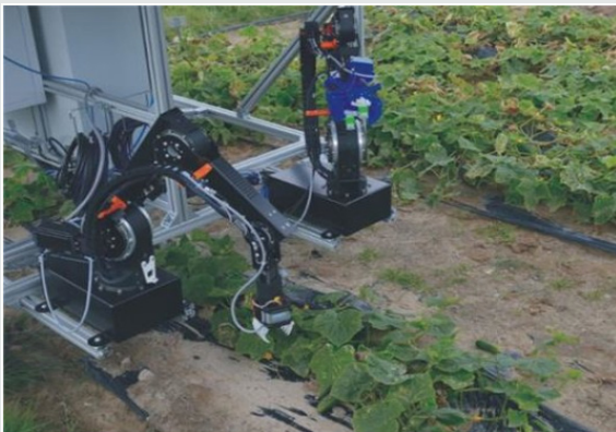
Figure 3: Illustrates prototype of the dual-arm robot system during the first field tests. Image Credit: Fraunhofer IPK [3].
