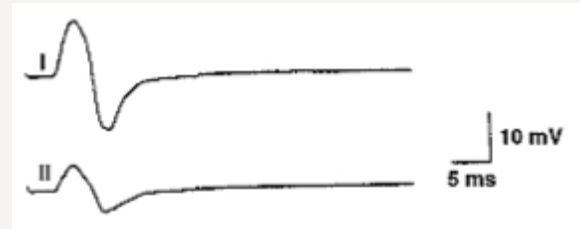
Figure 5: The active and reference pickup should not be too close together. Effect on the amplitude of varying the inter-electrode separation.
