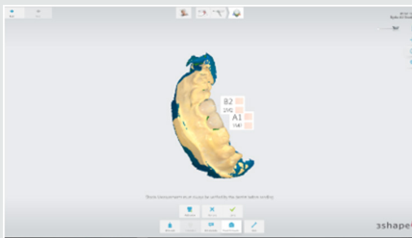
Figure 3: Demonstrated the color shade measurement of the abutment and pontic portions of the acrylic bridge.
