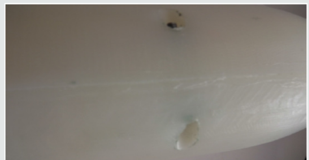
Figure 13: External groove sealing using silicon-based glue.
