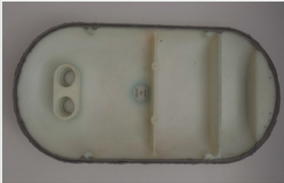
Figure 8: Use of Gasket Maker paste to customize sealing.
