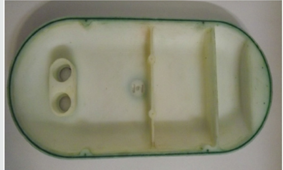
Figure 11: Body groove filled with grease.
