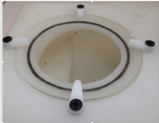
Figure 16: Valve opening: sealing with O-ring groove.
