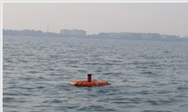
Figure 1: Deployment of Aquadopp 2MHz current meter in the coastal water.
