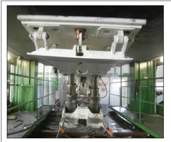
Figure 1: Prototype section of the powered roof support during bench tests.
