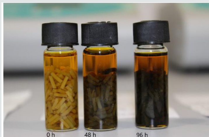
Figure 3: TLC propellant sample without artificial aging (0 h = current state of propellant), and after aging on 80°C in periods of 48 h (2.3 year) and 96 h (4.6 years).
