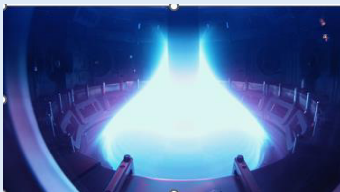
Figure-3: Hot Plasma, Magnetically Confined in a Tokamak (Source: U.S. Department of Energy).
