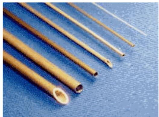
**Figure 6:** Different Sizes of NiTiNol Tubes.
