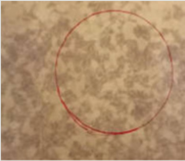
Plate 7: A1 Welded Zone Annealed at 650.
