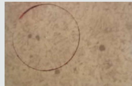
Plate 12: A2 - Welded Zone Control Sample (X250).
