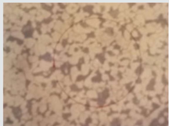
Plate 5: A1 Welded Zone Annealed at 450°C(X250).
