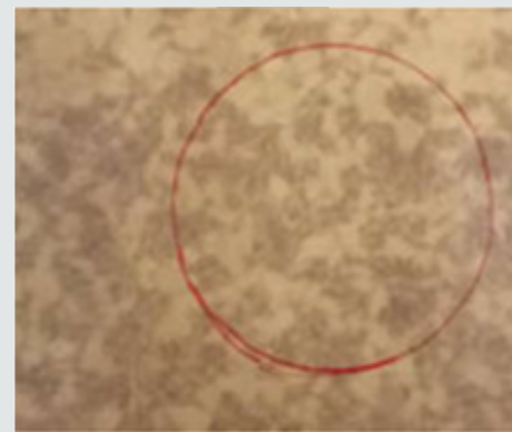
Plate 11: HAZ Annealed at 750 °C(X250).
