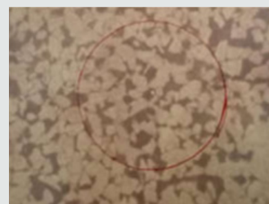
Plate 13: HAZ Control Sample (X250).
