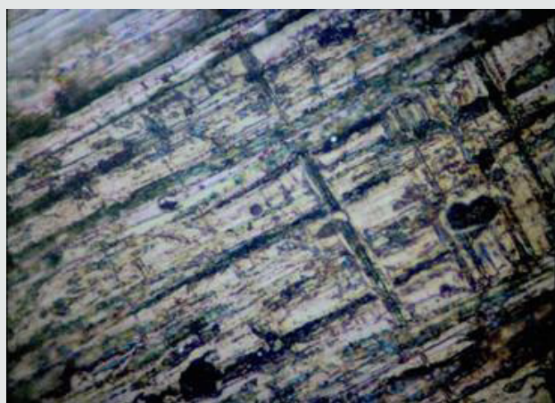
Figure 2: Microscopic image of the surface of a reference (untreated or unpolished) sample at x100
