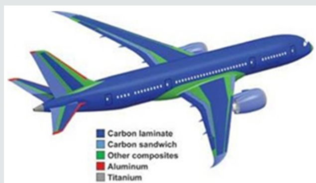
Figure 5: Composition of composites in B787 Dreamliner.
