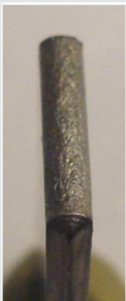
Figure 4: Fully bent specimen before heat treatment (bending angle of 180^{\circ} ).
