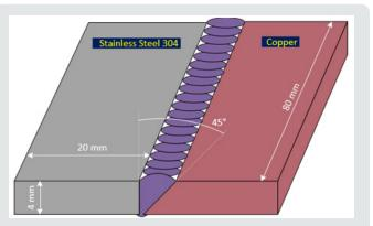
Figure 1: Schematic of joint design (units are in mm).
