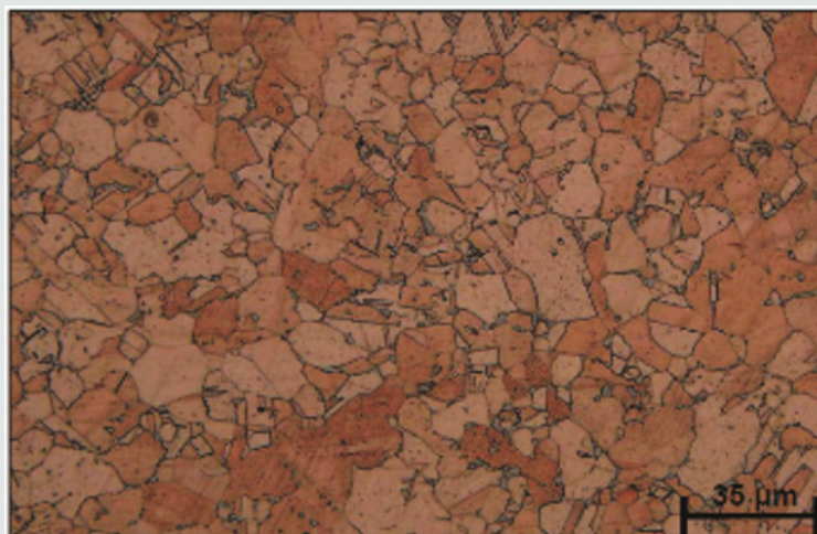
Figure 7: Microstructure of Cu-Sn-Bi alloy as revealed by optical microscopy. Etchant: FeCl 3 and HCl in ethanol.
