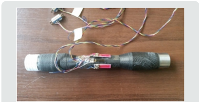
Figure 3: Element of an oil pipeline with strain gauges.
