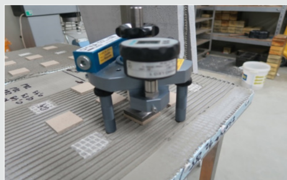
Figure 1: Measuring stand DYNA Z16 Leo1 for the pull-off method.
