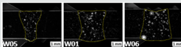
Figure 6: LOM images showing porosity content of welds produced using 1100W (W05), 2200W (W01) and 3400W (W06). The yellow contour shows the fusion zone. The fusion zone and area fraction pores increased with increasing power.
