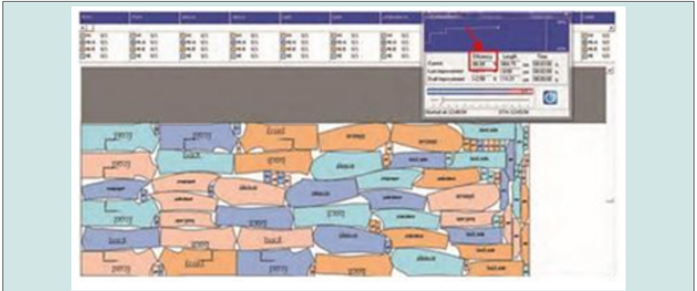
Figure 1: A marker plan with 4 graded size patterns showing efficiency of 86.89% [3].
