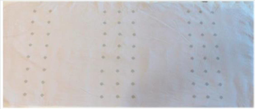
Figure 7: The e-textile mat with the embroidered textile sensors.
