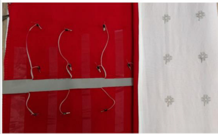
Figure 8: The reverse side of the e-textile mat with the embroidered textile sensors.
