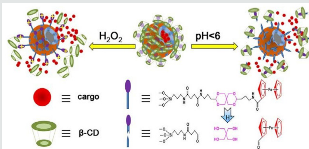
Figure 7: Schematic diagram of the release of R6G from mechanized HMSNs-S1 [18].
