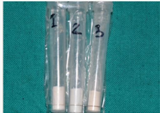
Figure 4: Materials in plastic caps (1) Chalk dust, (2) TCP and (3) Egg-shell.
