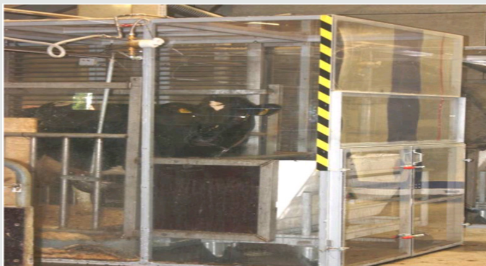
Figure 3: Open Circuit Chambers [1].
