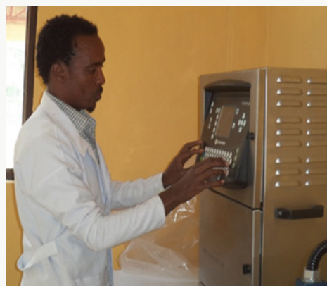
Figure 14: Printing of mini straws using a computerised machine, domino.
