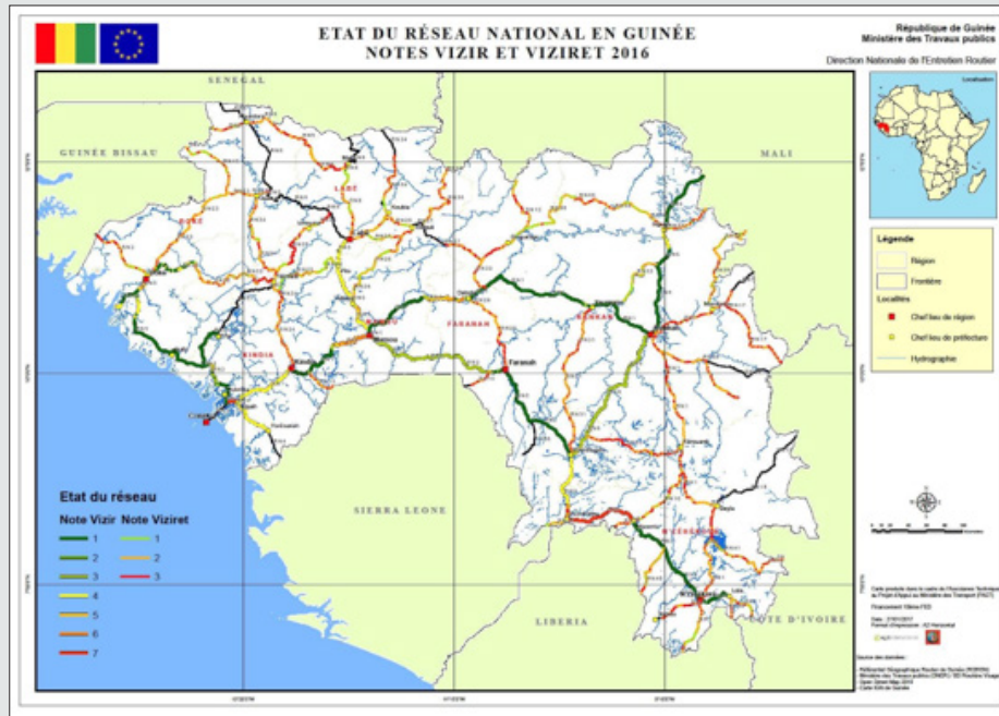
Figure 3: Surface condition and degradation of Guinean roads (Viziroad notes) in May 2016.
