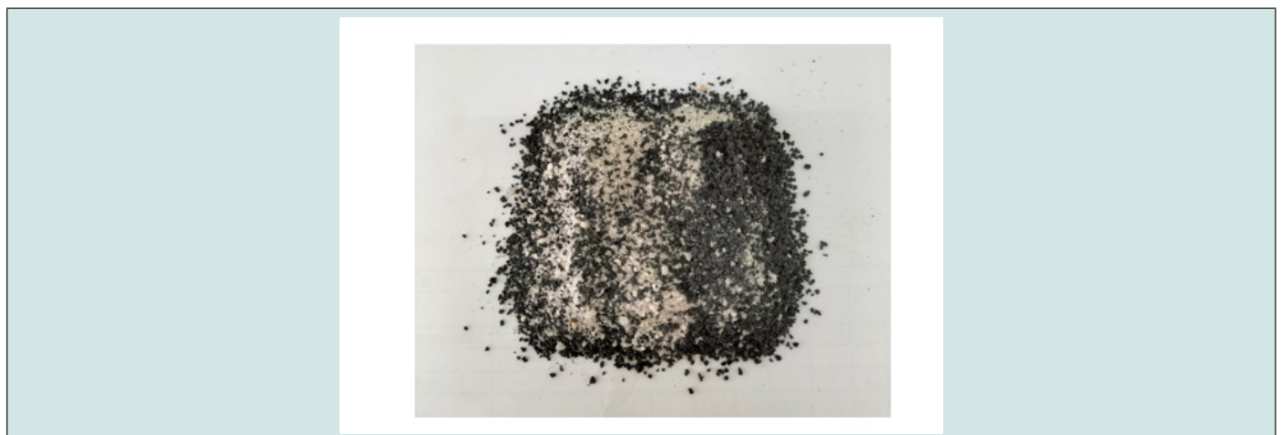
Figure 3: Sand mixed with granulated waste rubber
