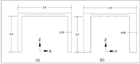
Figure 5: Columns Dimensions in meters: (a) Front view, (b) Side view.
