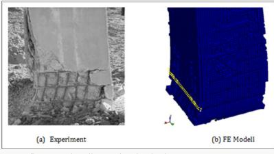
Figure 2: Modell Verification, Deflection and Spalling under Blast loading.
