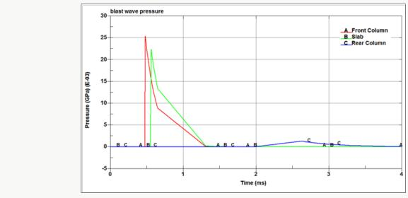
Figure 9: External blast wave pressure on structure.
