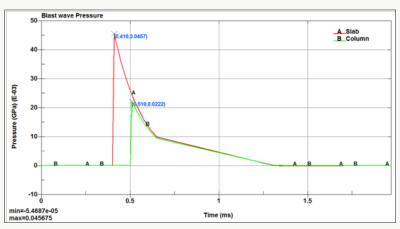
Figure 6: Blast wave pressure on slab and columns.
