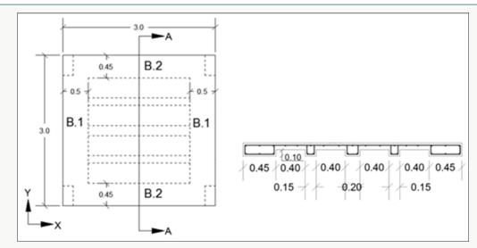
Figure 4: Slab dimensions and reinforcement details.
