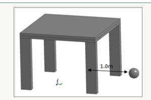
**Figure 8:** Schematic of the structure and the location of external explosion.
