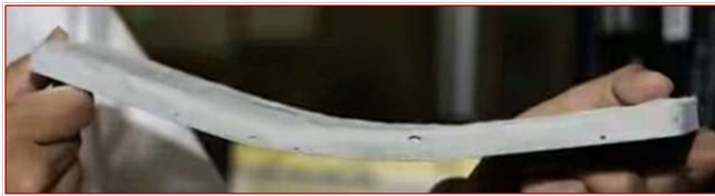
Figure 1: Flexible concrete specimen made by Professor Victor Li.
