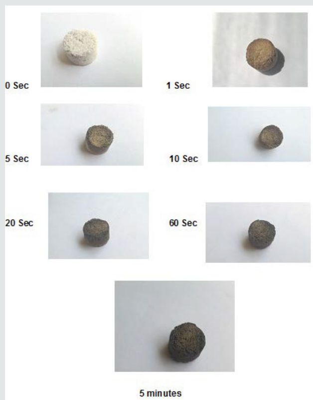
Figure 10: Effect of H 2 S gas on a porous glass pellet exposed to different periods.
