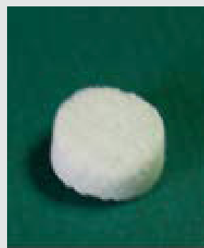
Figure 1: A glass pellet prepared from very fine glass grains (- 0.075mm).
