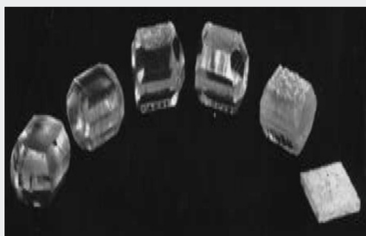
Figure 13: Crystals grown in the presence of increasing concentrations of aluminum. Aluminum by weight of quartz nutrient: (1) 0.05%, (2) 0.125%, (3) 0.25%, (4) 0.50%, (5) 1.25%, and (6) 2.50%.
