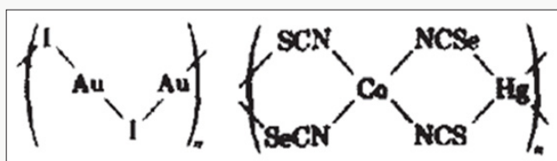
Figure 8a: Coordinating polymer formed from monodentate halide or pseudohalide ligands.
