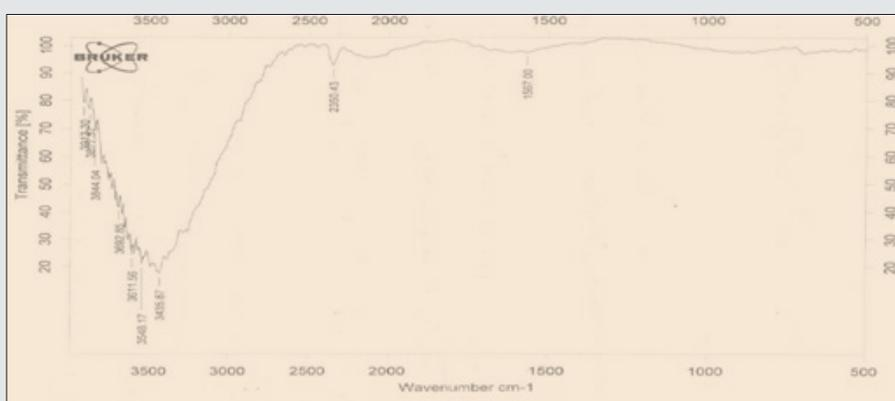
Figure 1: Fourier transformation of the infrared spectrum of carbon nanotubes before absorption.
