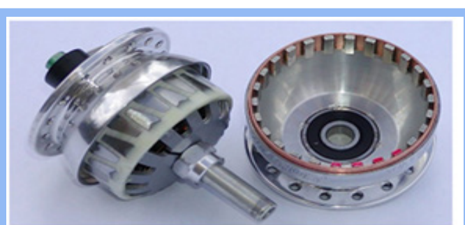
Figure 32: Mechanism of a xero dynamo wheel set generator.
