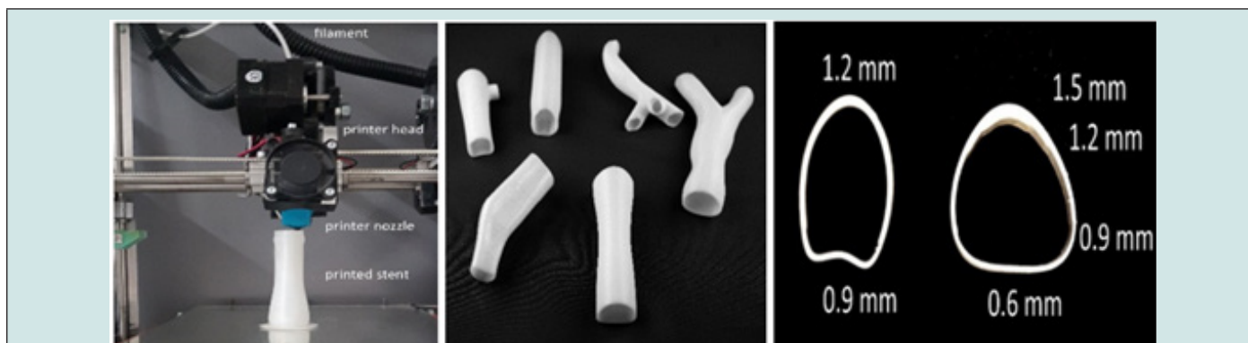
Figure 2: Stents are printed from flexible polymer filaments with a modified 3 D printer. Stent wall thickness can be varied influencing the local recoil and dynamic behavior.
