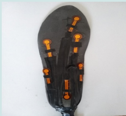
Figure 10: Sensor Placement in the sole.
