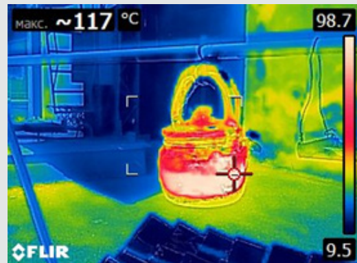
Figure 4: Temperature field on the teapot located in the focal zone of the multi-facet helio kitchen .
