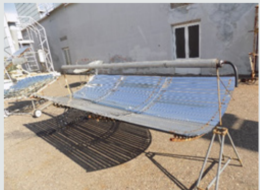
Figure 6: Solar kitchen, consisting of a cardboard concentrator covered with reflective foil .
