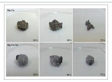
Figure 2: Visual comparison of samples Mg-40Ca and Mg-Ca-Gd at 24, 48 and 72 hours of immersion in NaCl at 36°C.
