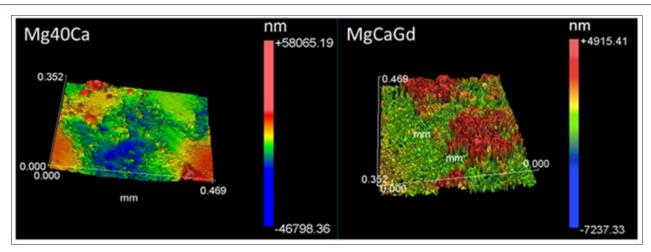
Figure 4: Tridimensional representation of surface morphology after corrosion of Mg40Ca alloy (left) and Mg-Ca-Gd (right).
