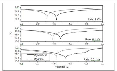
**Figure 1:** Potentiodynamic polarization curves acquired at a rate of 1, 0.1 and 0.01 V/s. Samples were immersed in NaCl 0.9% solution at 37°C and pH=7.4. Electrodes were stabilized for 1 hour before data acquisition.
