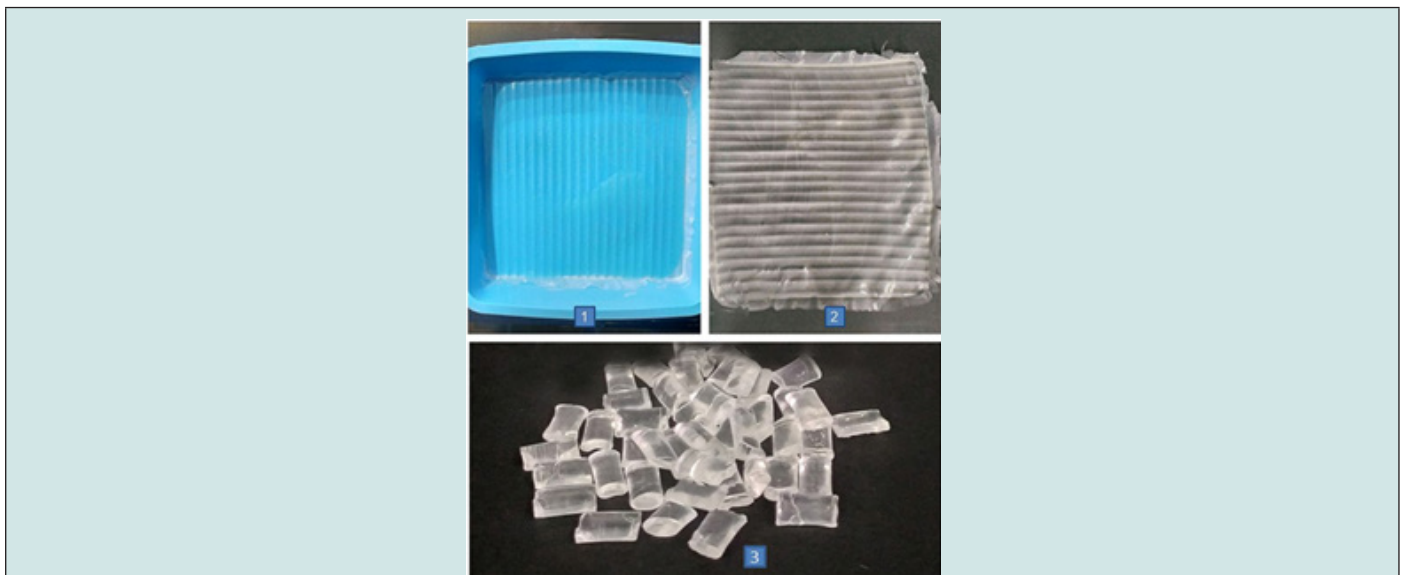
Figure 3: Obtention of Paraloid B72® sheets (preparation in mould 1-2 and final product 3).
