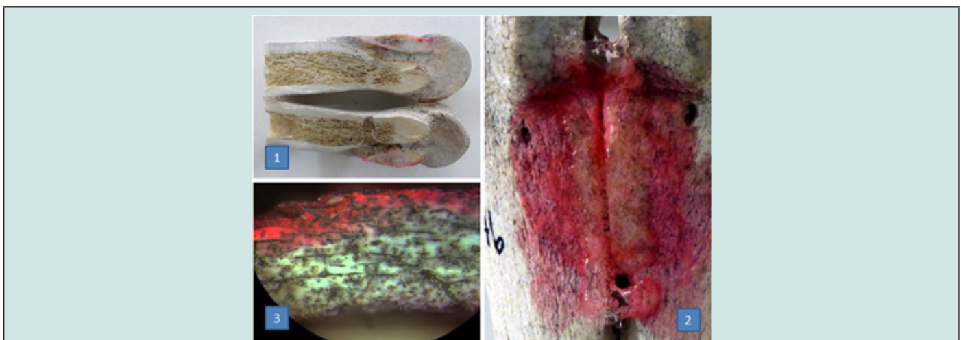
Figure 11: Type 1 samples (deer metapods), detail of staining after removing a Paraloid B-72® sheet (1,2) and study of penetration capacity by marking with 50x safranin (3).
