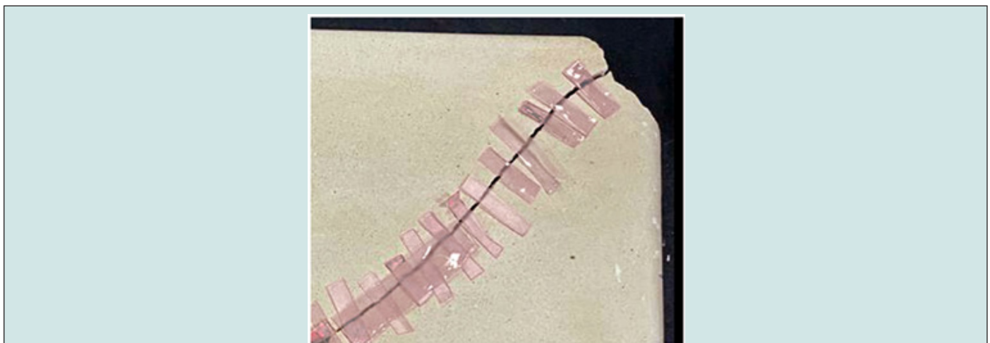
Figure 9: Application of Paraloid B-72® sheets in a fissure (type 4 samples).
