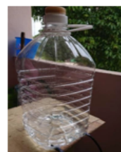
The tanks are from used cooking oil bottle and is washed with soapy waterand tap water until is clean from oil trace.
