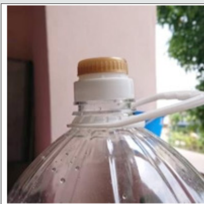
Figure 7: When the cap is closed, no atmospheric pressure is present, stopping the flow of water.
