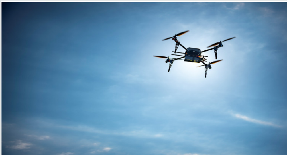
Figure 4: Fox's 650 Class Quad Copter is nicknamed Surely. Surely carries two sensors: a) Goodness, a MicaSense RedEdge® multispectral sensor and b) Mercy, a Canon SX 260 RGB camera.
